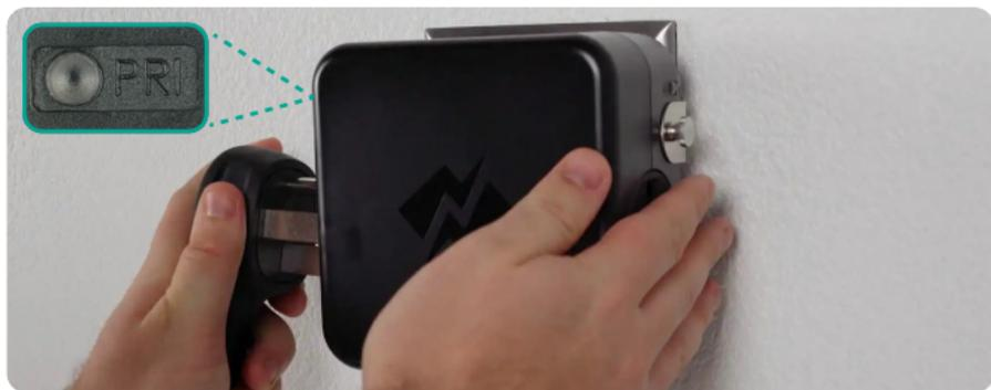
The device plugged in to the Primary side will always take priority over the device plugged into the Secondary side. This is typically your appliance, or if charging two EVs, the Primary should be the EV you want to charge first.
