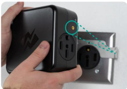
Unscrew the corresponding screws from the faceplate, then screw in the bracket using the bracket screws (2x) so the mounting bracket is flush with the faceplate.
